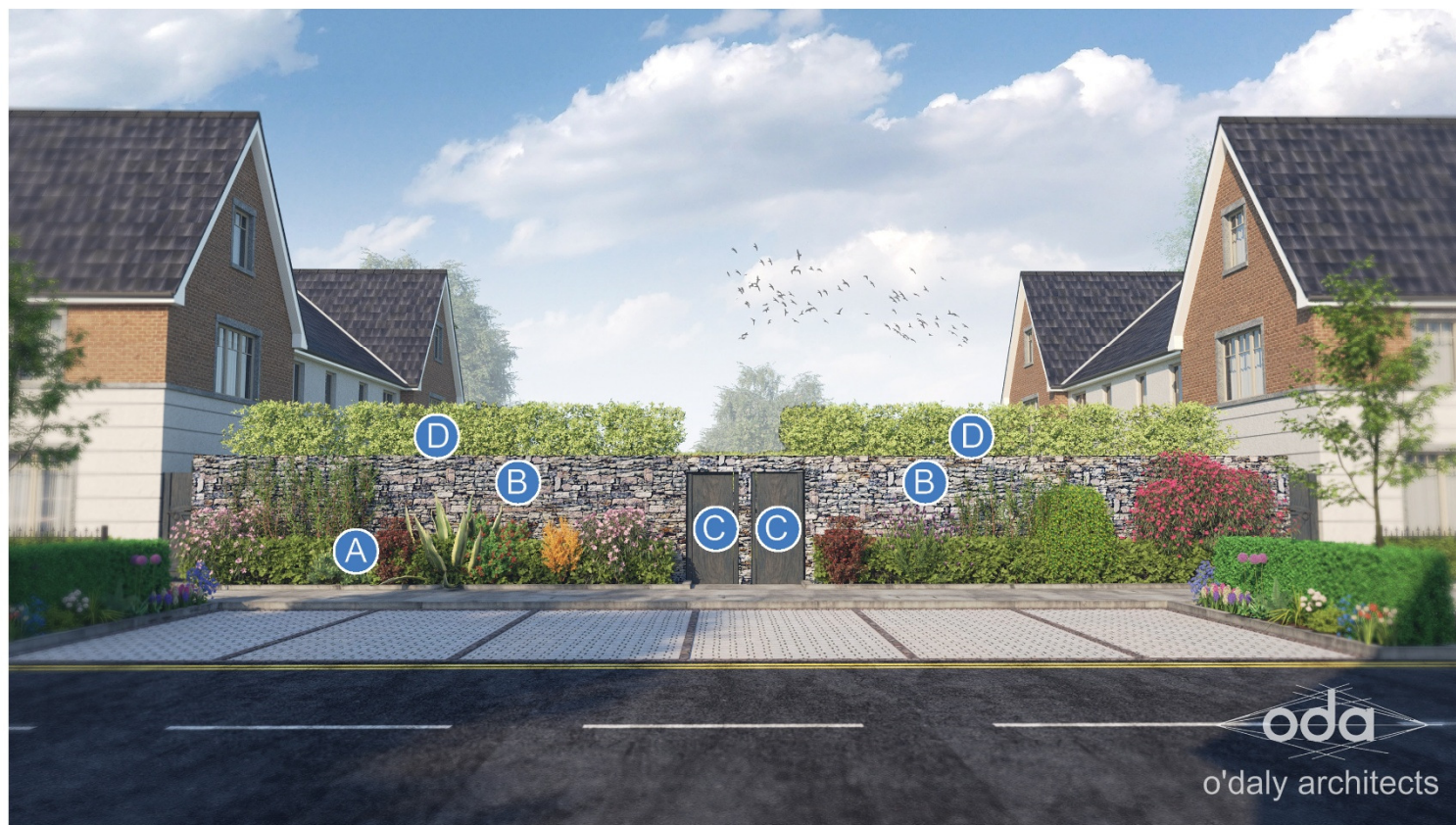
Fig. 17 – Proposed boundary treatment between dual frontage house private gardens and Western side of subject site (facing into scheme). Mid-terrace garden access doors are proposed on this side (each door only serves max. 2 gardens).
